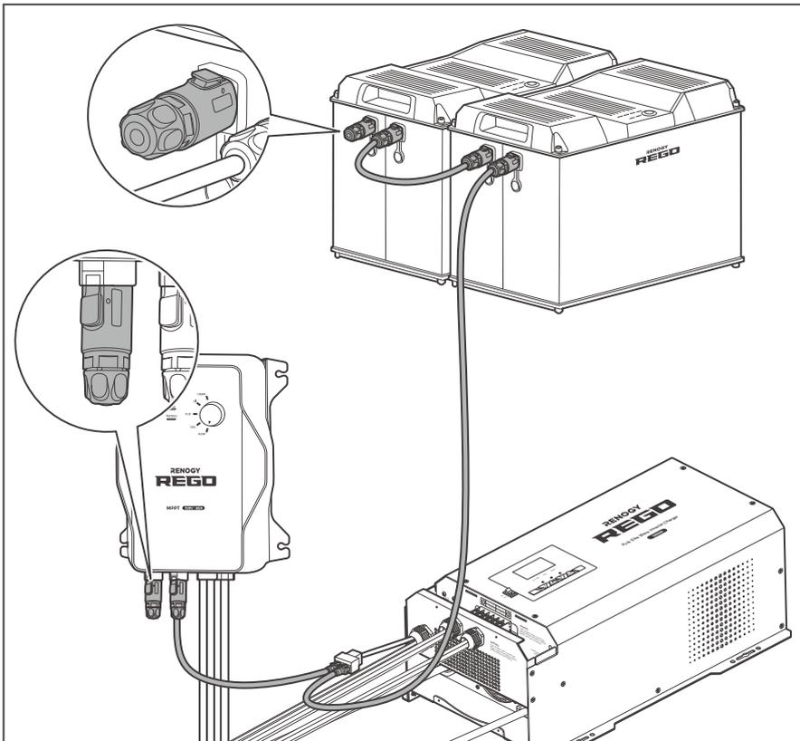
4. Connect the other ends of the LP16 Plug (7-Pin) to RJ45 Communication Adapter Cables to the vacant CAN communication ports of other REGO devices. Insert the terminal plugs (sold separately) into the vacant CAN communication port of the first and last REGO devices.
