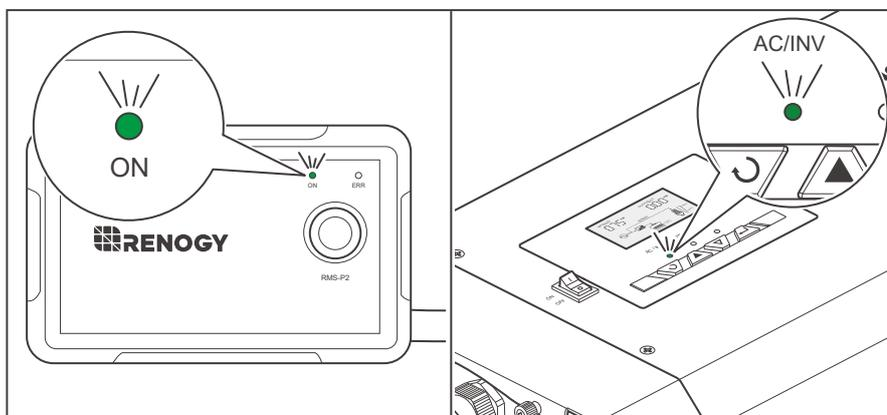
1. The ON indicator of the wired remote control and the AC/INV indicator of the inverter charger flash green when the inverter charger is powering loads from the battery.
