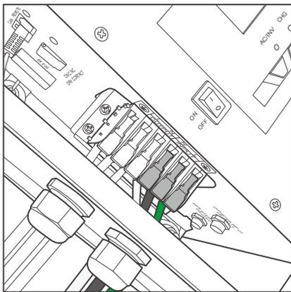
4. Press down the switch of the harness retainer of the AC Input Lever Terminal Block.
