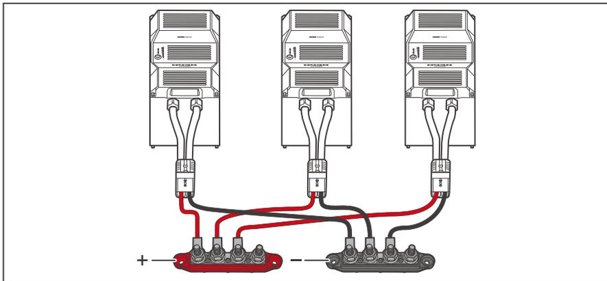
2. Connect the positive and negative ring terminals of the Adapter Cables to the Positive and Negative Busbars (not included) respectively.
