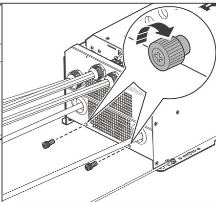
2. Install the DC Cable Plate and drive the two panel screws clockwise to fix the plate.
