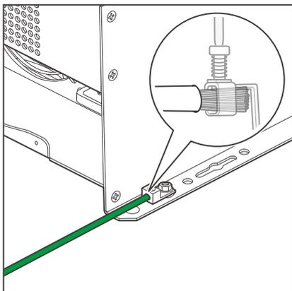
2. Insert one end of the bare wire into the wiring hole of the Chassis Ground Lug.
