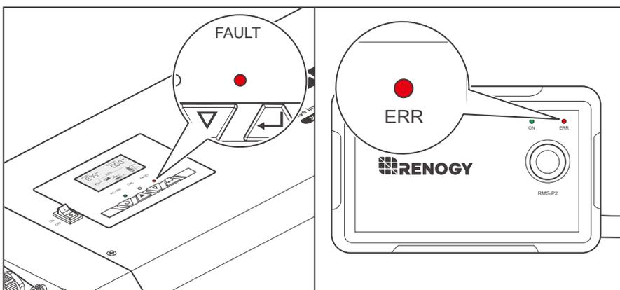
6. If both the FAULT and ERR indicators are always in red, and the buzzer sounds long, it means that the inverter charger needs troubleshooting. For details, refer to [Warning/Fault Codes](#) in this user manual. For more technical instructions, contact our customer service through [renogy.com/contact-us/](https://renogy.com/contact-us/).
