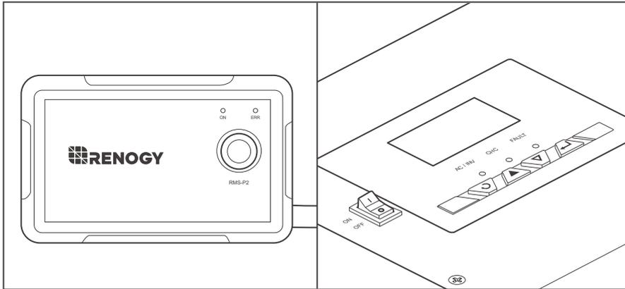
2. The LCD and LED indicators of the inverter charger as well as the ON indicator of the wired remote control go off when the inverter charger is powered off.
