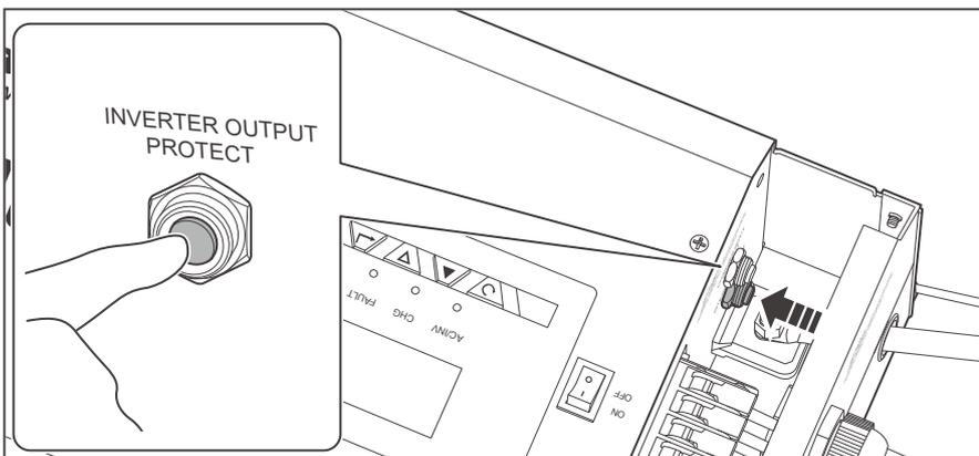
3. When the AC output current exceeds 30A, the Output Circuit Breaker will automatically pop out. Press the INVERTER OUTPUT PROTECT button to reset the circuit breaker.
