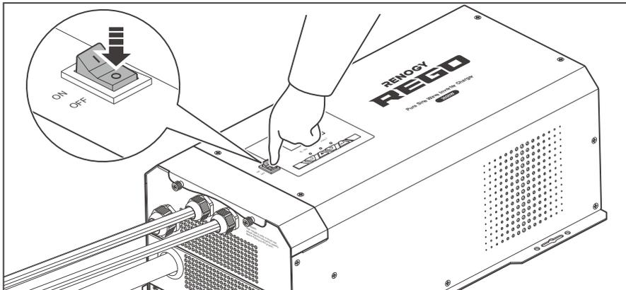
1. If you use the wired remote control, please turn the main switch of the inverter charger to "OFF" first.
