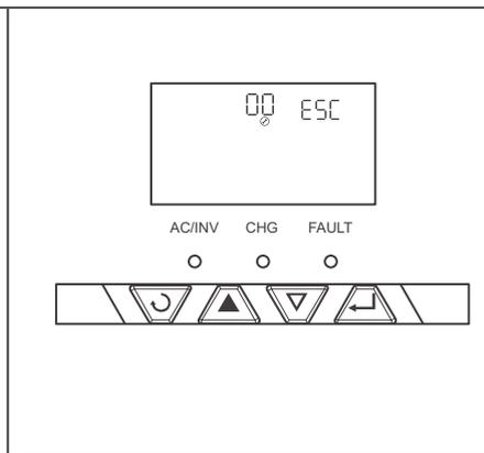
17. Long press  $\rightarrow$  until the LCD enters the setting mode.
