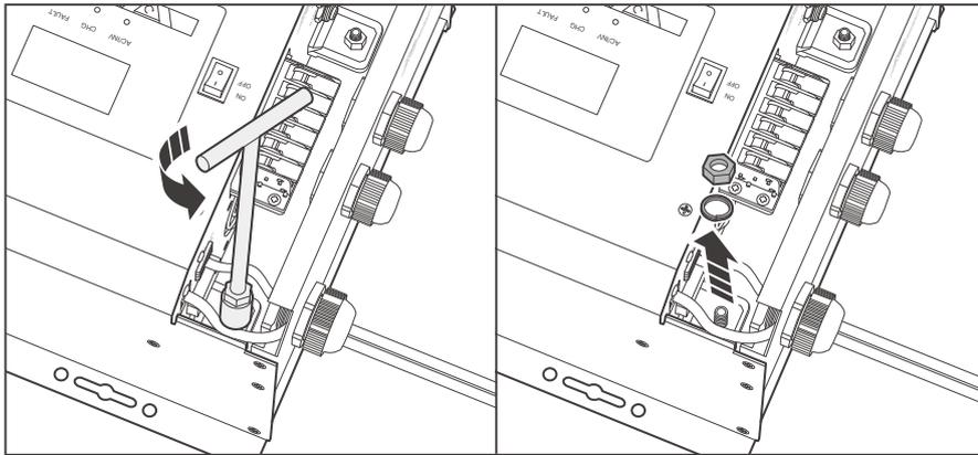
1. Remove the retaining nut of the DC Negative Battery Terminal by turning it counterclockwise with a socket wrench and then remove the gasket.
