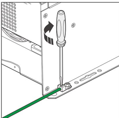
3. Tighten the cable retainer screws for the Chassis Ground Lug clockwise with a slotted screwdriver to fasten the cable.
