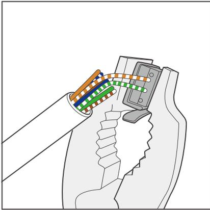
4. Squeeze the crimp areas of the Drop Plugs with the Split Joint Pliers.
