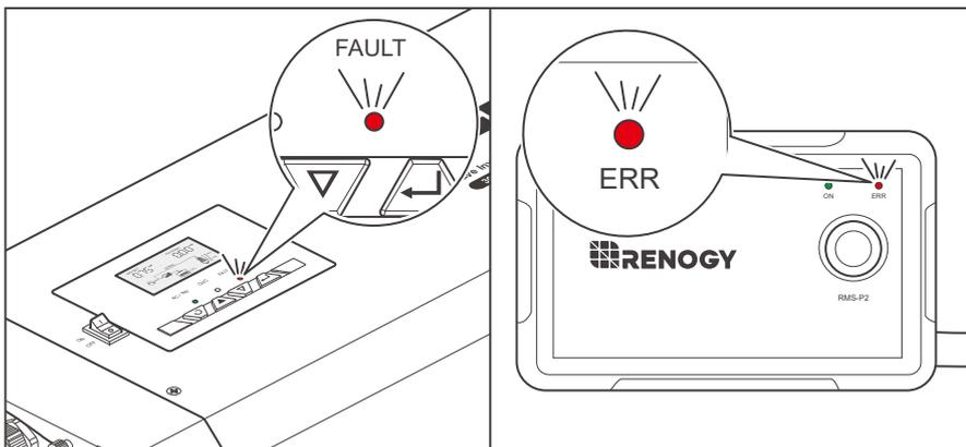
5. If both the FAULT and ERR indicators flash red, and the buzzer sounds at the same time (0.5s), it means warnings are provided by the inverter charger. For details, refer to [Warning/Fault Codes](#) in this user manual.
