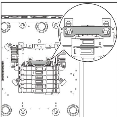
1. Remove the front cover of the AC load center and connect the two live wire busbars with a copper strip.
