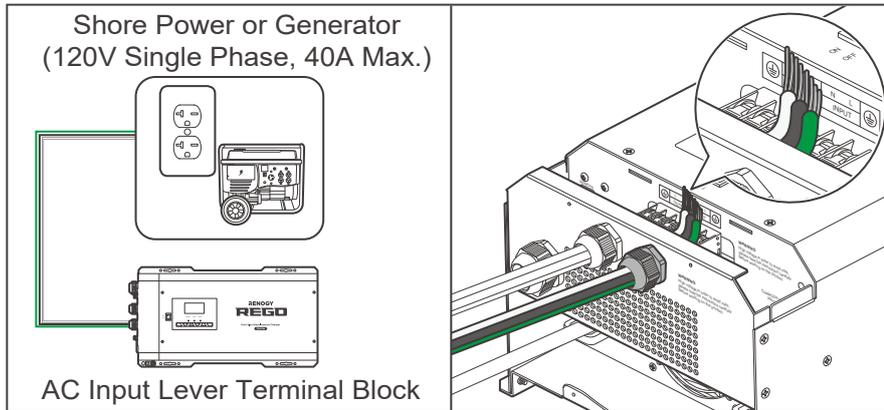
1. Run the AC power cable through the AC Input Cable Grommet.
