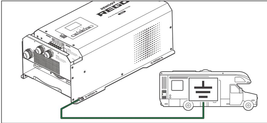
4. Connect the other end of the bare cable to the Chassis Ground Lug of the RV.
