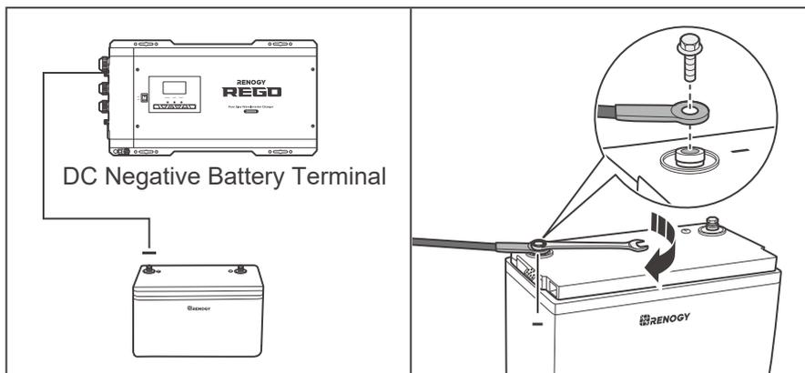
1. Connect the negative ring terminal to the negative terminal of a Normal Battery. Tighten the wire retaining bolt with a wrench.
