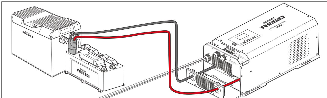
1. Connect the Anderson 350 connector of the battery adapter cable to the System Combiner Box.
