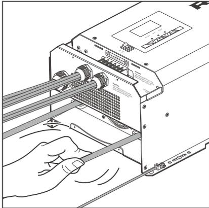
1. Check and make sure all cable connections are tight and secure.
