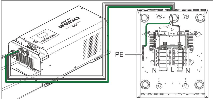
2. Connect the AC Output cable of the inverter charger to the AC load center. Connect the live wire to the (L) terminal, the neutral wire to the (N) terminal, and the ground wire to the (PE) busbar.
