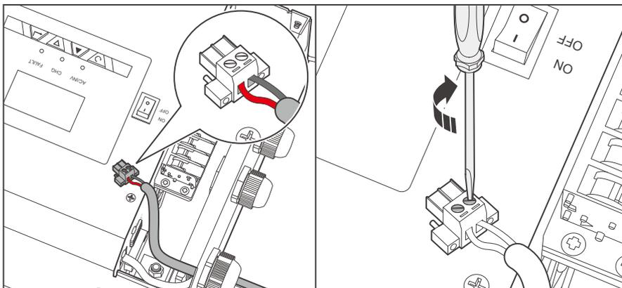
3. Insert the bare terminal of the temperature sensor into the harness connector and tighten it with a slotted screwdriver by turning the cable retainer screw for wire harness connector clockwise.
