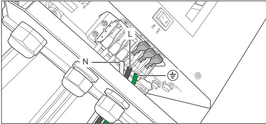
3. Connect the live wire to the (L) terminal, the neutral wire to the (N) terminal, and the ground wire to the (⊕) terminal.
