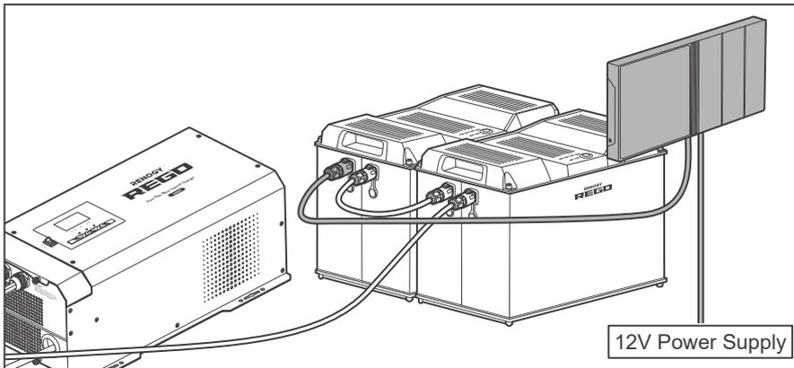
2. Connect the Renogy ONE to the free CAN Communication Port on the REGO device with the Communication Adapter Cable (sold separately).
