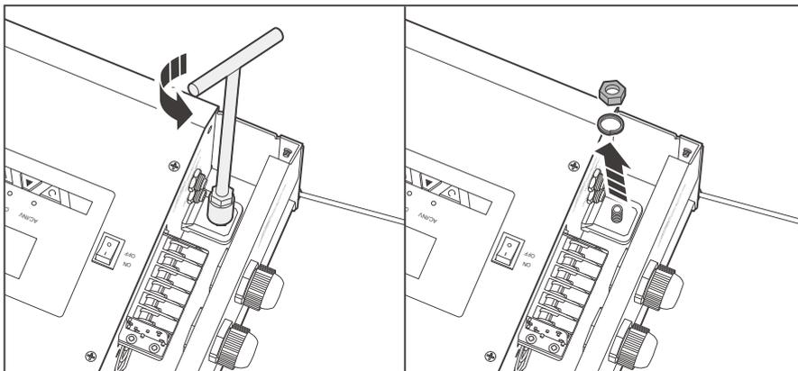
2. Remove the retaining nut of the DC Positive Battery Terminal by turning it counterclockwise with a socket wrench and then remove the gasket.
