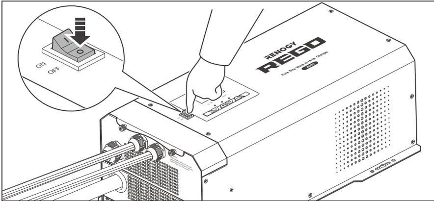
1. Press the main switch of the inverter charger to "OFF" to turn it off.
