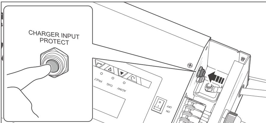
2. When the AC input current exceeds 40A, the Input Circuit Breaker will automatically pop out. Press the CHARGER INPUT PROTECT button to reset the circuit breaker.
