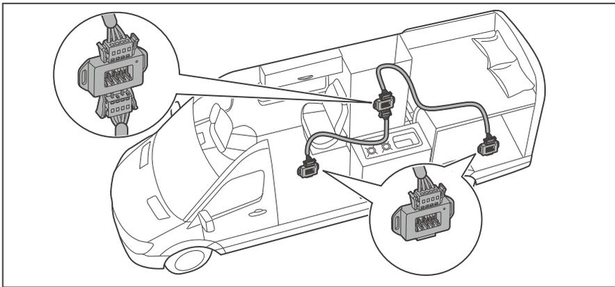
5. Locate the drop tap (not included) on the RV-C bus that is the closest to the installation site of the inverter charger. The drop taps are usually located above the entry door, in the bathroom, or under the bed in the RV.
