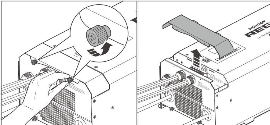
1. Turn the two upper panel screws counterclockwise by hand or a Phillips screwdriver, and remove the Top Plate.
