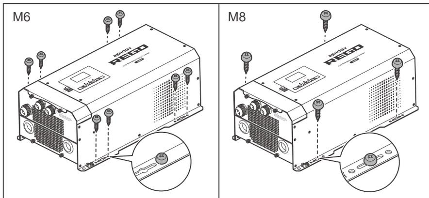
Align the inverter charger with the mounting position to fix it with self-tapping screws through the mounting holes.
