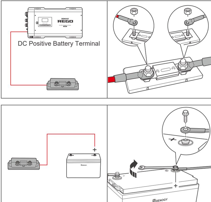
2. For your safety, it is recommended to use a DC fuse (400A). Connect the positive ring terminal of the inverter charger adapter cable to the DC fuse. Install the fuse wire on the other end of the fuse.
