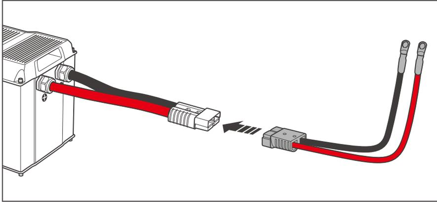
1. Connect the Anderson Connectors of the batteries to the Adapter Cables (sold separately).
