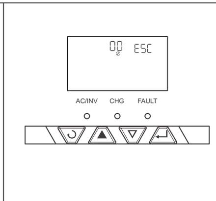
6. Long press ← until the LCD enters the setting mode.
