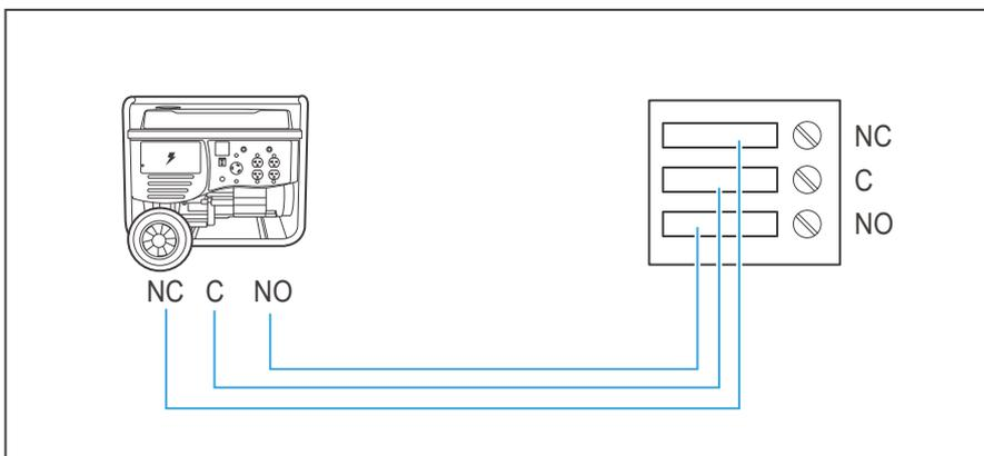
5. Connect three signal lines to the corresponding NC, C, and NO wiring holes.
