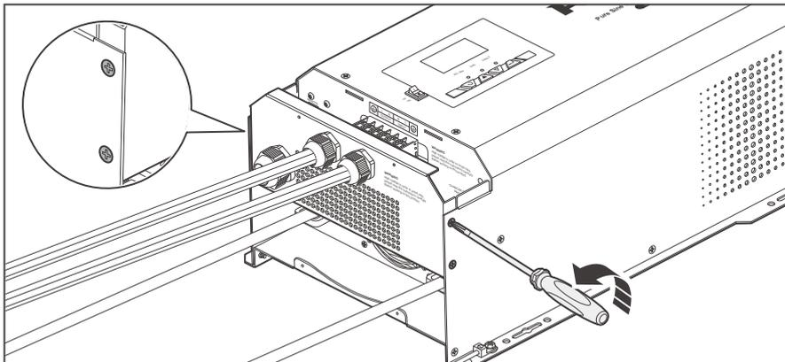
1. Remove four retaining nuts of the AC Cable & Accessory Plate by turning them counterclockwise with a Phillips screwdriver.
