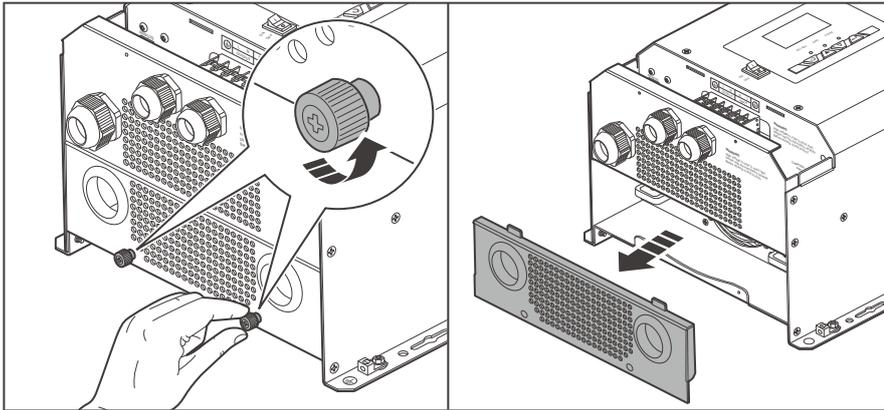
2. Turn the two screws on the lower panel counterclockwise by hand or a Phillips screwdriver, and remove the DC Cable Plate.
