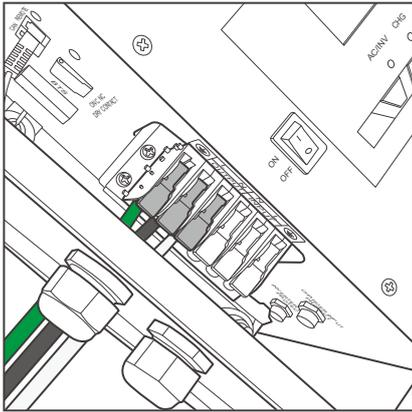
4. Press down the wire harness retainer of the AC Output Lever Terminal Block.
