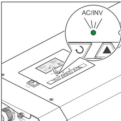
2. The screen lights up and displays the status after the inverter charger is powered on. The AC/INV indicator will light up based on the usage.
