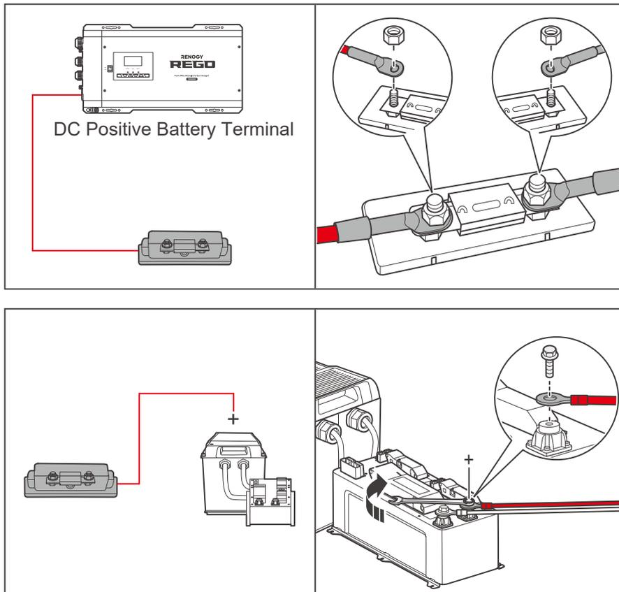
2. For your safety, it is recommended to use a DC fuse (400A). Connect the positive ring terminal to the DC fuse. Install the fuse cable on the other end of the fuse.
