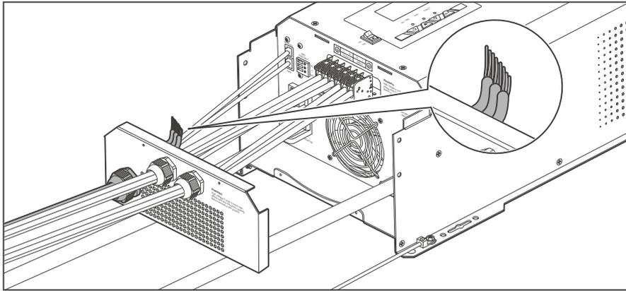
3. Run three signal lines through the Remote & Accessory Cable Entry.
