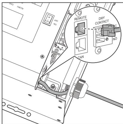
2. Connect the connector to the Wired Remote Port (REMOTE).
