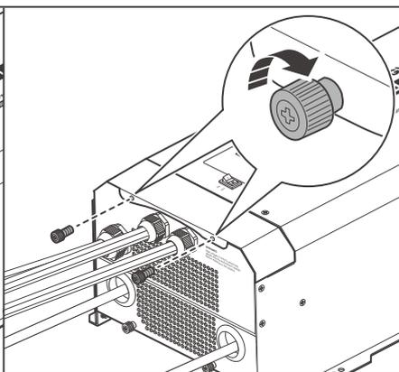
3. Install the Top Plate. Drive the two panel screws clockwise to fix the plate.
