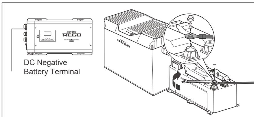
1. Connect the negative ring terminal to the negative terminal of the system hub. Tighten the wire retaining bolt with a wrench.
