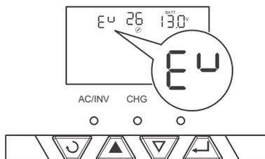
14. For lithium battery, set the maximum charging voltage in Program 26.
