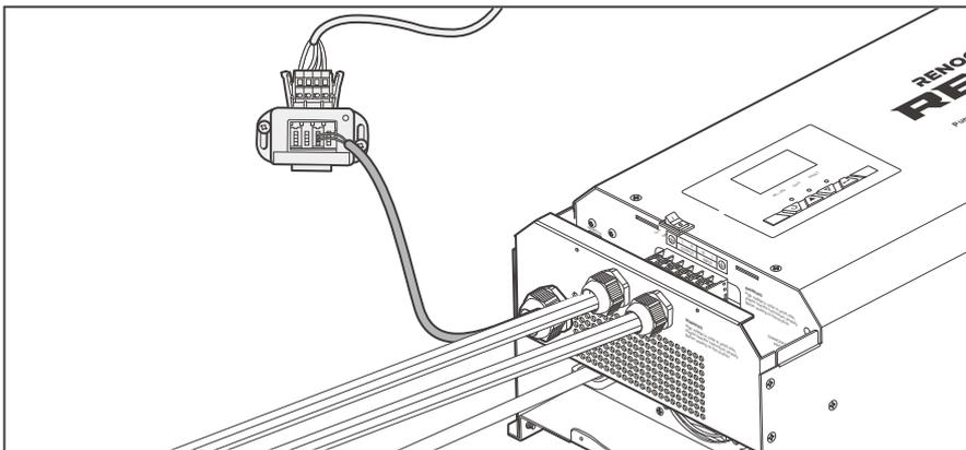
6. Connect the Drop Plugs on the drop cables and other REGO devices to the drop sockets on the drop tap.
