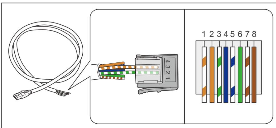
3. The white green CAN\_H wire goes to pin 2 and the white orange CAN\_L wire goes to pin 3. Leave pin 1 and pin 4 empty.
