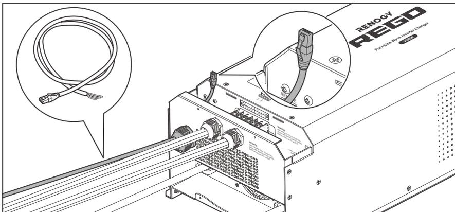
1. Insert the RJ45 connector of RJ45 Plug to the Bare Drop Cable through the Remote & Accessory Cable Entry.
