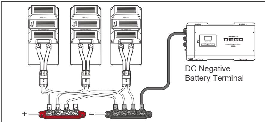
3. Attach the negative ring terminal to the Negative Busbar and tighten the wire retaining bolt with a wrench.
