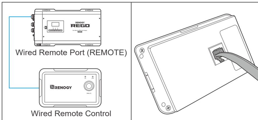
3. Connect the connector on the other end of the RJ11 cable to the Wired Remote Control.
