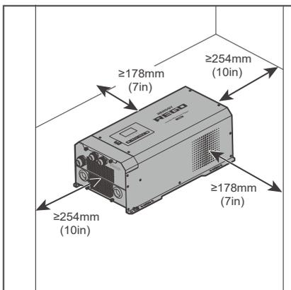
1. Ensure enough space to avoid tangles and kinks of cables. Allow at least 10 inches of clearance at the fan and at least 7 inches around each side. It is better to have a larger ventilation gap. Do not obstruct the fan openings.
