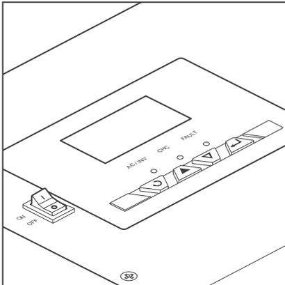
2. The LCD and the LED indicators go out when the inverter charger is powered off.
