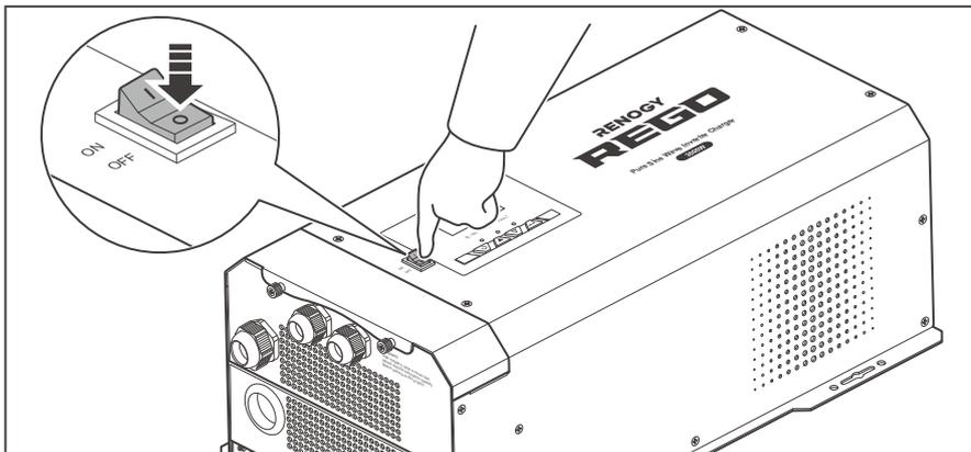
3. After the installation site is determined, rock the main switch of the inverter charger to the "OFF" position and keep it until the inverter charger is ready to be powered on.
