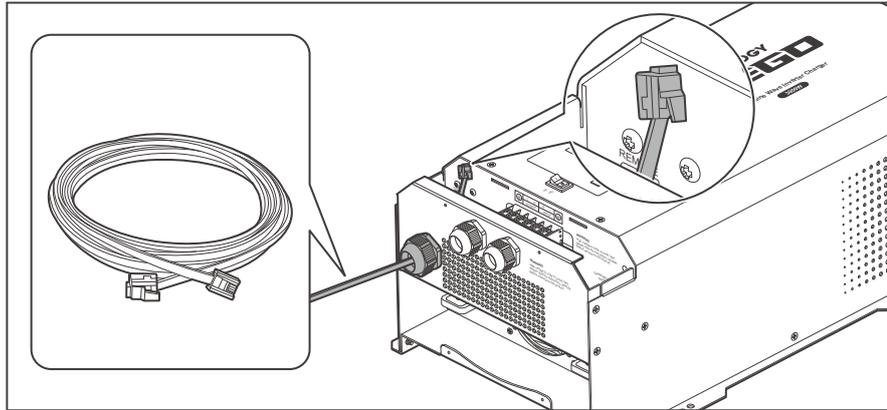
1. Run one end of the included RJ11 cable through the Remote & Accessory Cable Entry.
