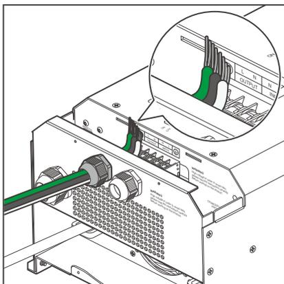
1. Run three bare wires through the AC Output Lever Terminal Block.
