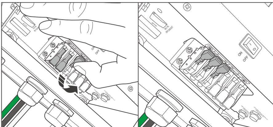
2. Push up the switches of the wire harness retainer of the AC Output Lever Terminal Block.
