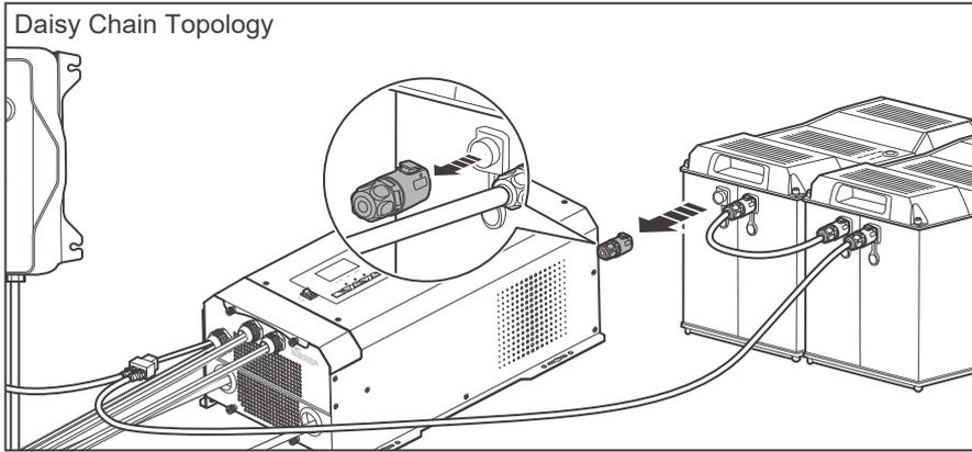
1. Remove the Terminator Plug from the REGO device at either end of the daisy chain.
