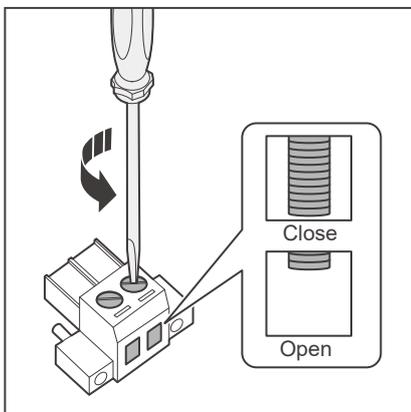
2. Turn the cable retainer screws for wire harness connector counterclockwise with a slotted screwdriver to ensure that the cable retainer is open.
