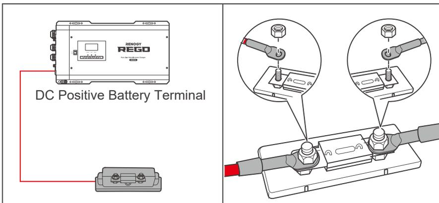
4. For your safety, it is recommended to use a DC fuse (400A). Connect the positive ring terminal to the DC fuse. Install the fuse wire on the other end of the fuse.
