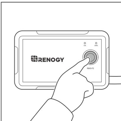
1. When using a wired remote control, press the button on the wired remote control to turn off the power.
