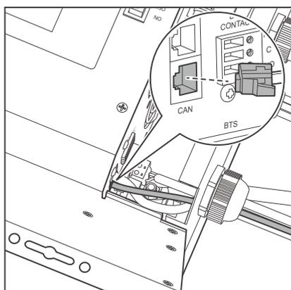
2. Connect the RJ45 connector to the Communication Port (CAN Bus).
