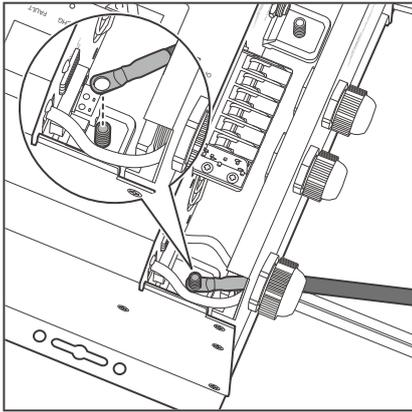
4. Connect the negative ring terminal to the DC Negative Battery Terminal.
