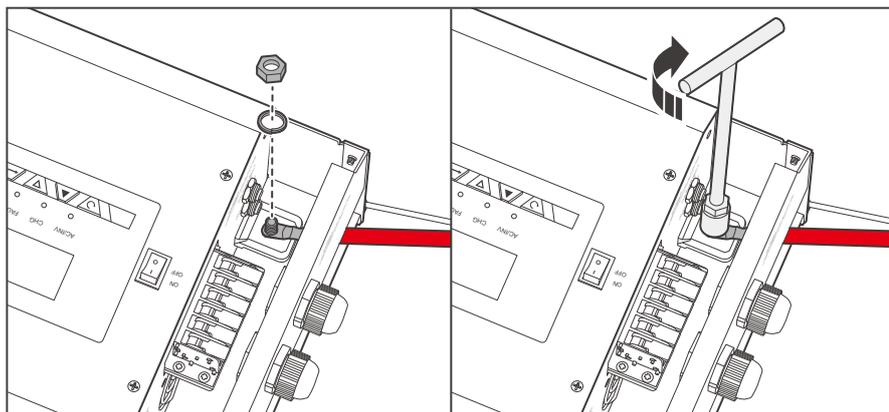
7. Install the gasket and retaining nut, and tighten the nut clockwise with a socket wrench.
