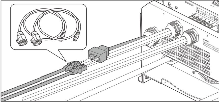
3. Connect the two RJ45 connectors of LP16 Plug (7-Pin) to the RJ45 Communication Adapter Cables to the RJ45 Network 1 to 2 Port Ethernet Adapter Splitter.
