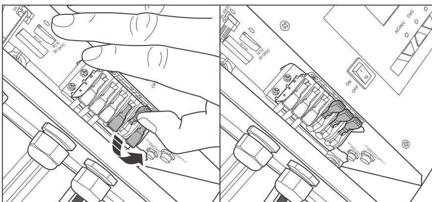
2. Push up on the lever of the AC Input Terminal Block.
