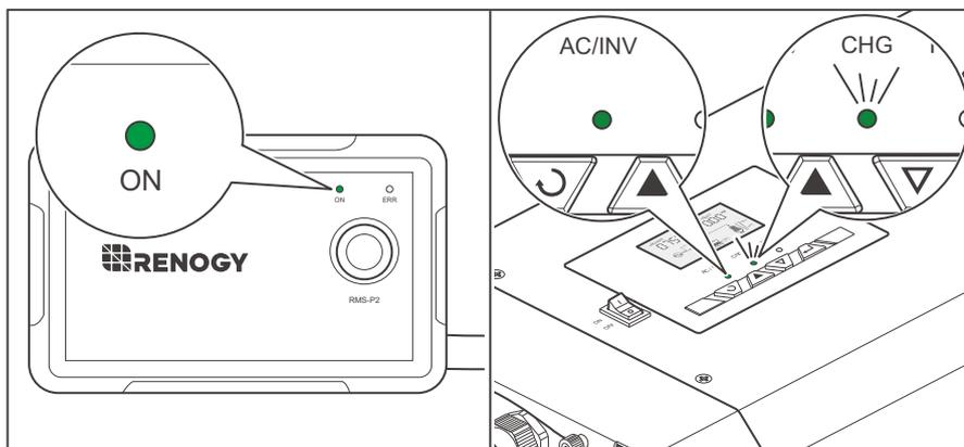
2. The ON indicator of the wired remote control and the AC/INV indicator of the inverter charger are solid green when the inverter charger is powering the loads through an AC Input Source, and when the inverter charger starts to charge the battery at the same time. The CHG indicator flashes green.
