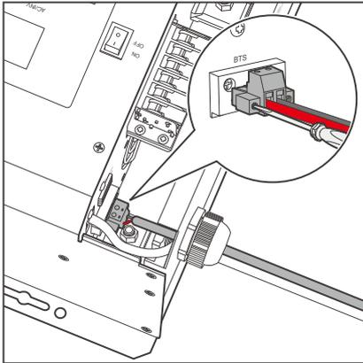
4. Plug the harness connector into the BTS Port of the inverter charger.
