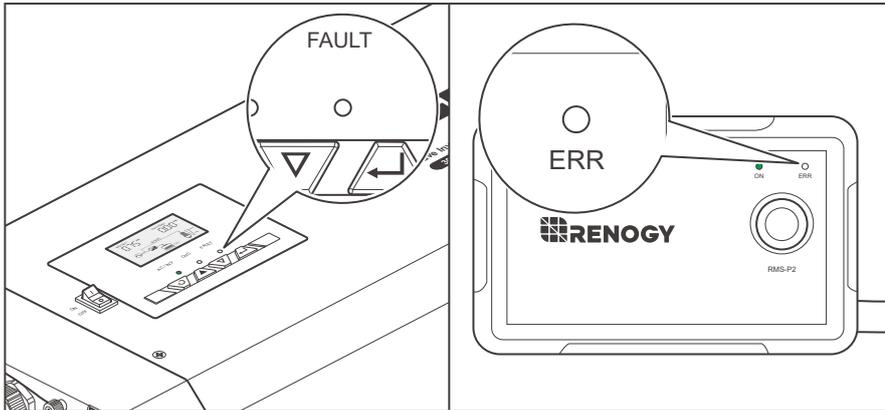
4. Under normal conditions, FAULT indicator of the inverter charger and the ERR indicator of the wired remote control will not light up.
