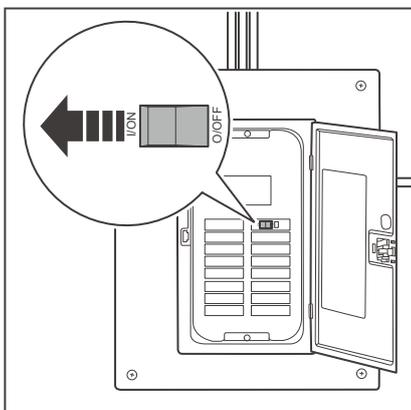
4. Install the front cover of the AC load center and turn on all the circuit breakers in the AC load center.
