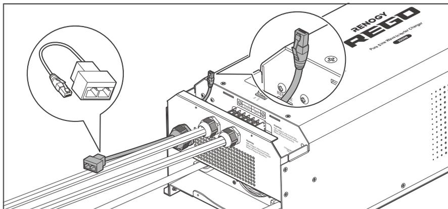
1. Insert the RJ45 connector of RJ45 Network 1 to 2 Port Ethernet Adapter Splitter through the Remote & Accessory Cable Entry.
