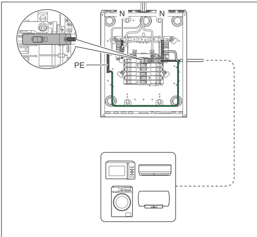
3. Select an appropriate circuit breaker according to the operating load current, and connect the load to the AC load center. Connect the live wire to the (L) terminal, the neutral wire to the (N) terminal, and the ground wire to the (PE) busbar.
