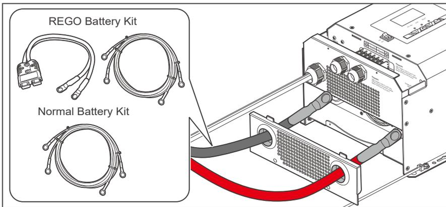
3. Insert the positive ring terminal of the battery adapter cable through the DC Positive Battery Cable Entry, and the negative ring terminal through the DC Negative Battery Cable Entry.
