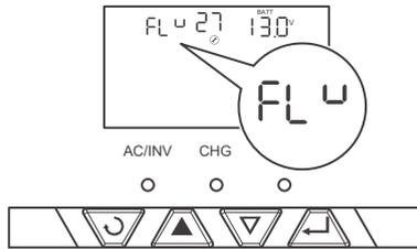
20. For lithium battery, set the battery low voltage open charging in Program 27.
