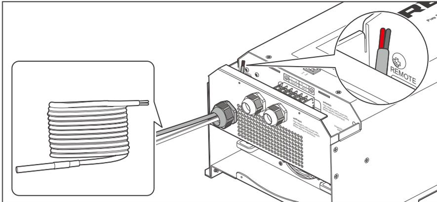
1. Run the bare terminal of the temperature sensor through the Remote & Accessory Cable Entry.
