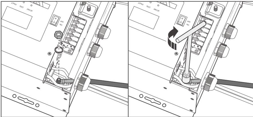
5. Install the gasket and the retaining nut, and tighten the nut clockwise with a socket wrench.
