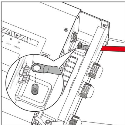
6. Connect the positive ring terminal to the DC Positive Battery Cable Entry.
