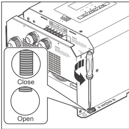
1. Turn the cable retainer screws for the Chassis Ground Lug counterclockwise with a slotted screwdriver to ensure that the cable retainer is open.
