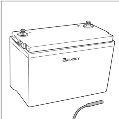
5. Place the temperature sensor near the battery and fix it with a cable tie or insulation tape if necessary.
