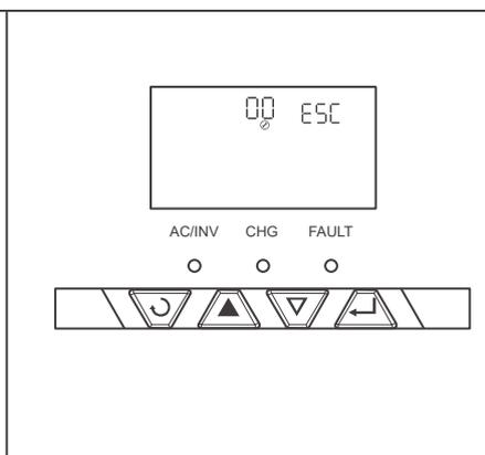
11. Long press  $\rightarrow$  until the LCD enters the setting mode.
