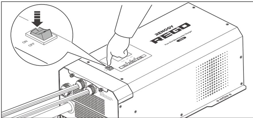
1. Press the main switch of the inverter charger to the "ON" position to power the inverter charger on.
