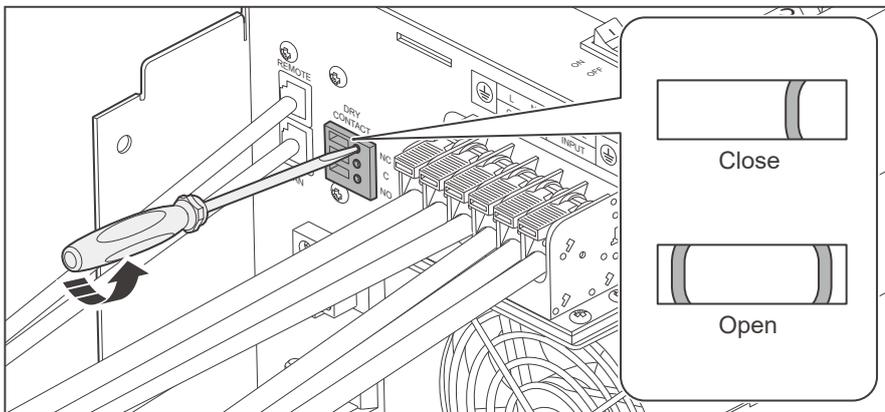
4. Turn the cable retainer screws of NC, C and NO of Dry Contact Relay Terminal Block counterclockwise with a slotted screwdriver to ensure that the cable retainers are open.
