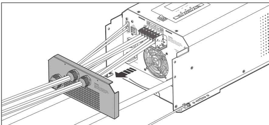
2. Remove the AC Cable & Accessory Plate.
