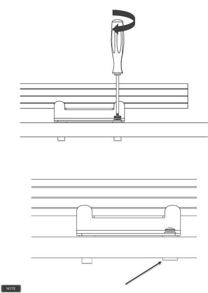
Screw has compressed and expanded the well nut, binding into the roof material.
