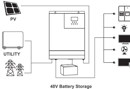
**Photovoltaic Modules (PV):** convert light energy into DC power, charge the battery through the solar inverter charger, or directly reverse into alternating current to power the load.
