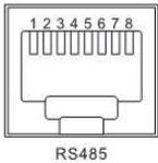
This port will be used for connecting to the BT-2 Accessory for remote monitoring and control.
