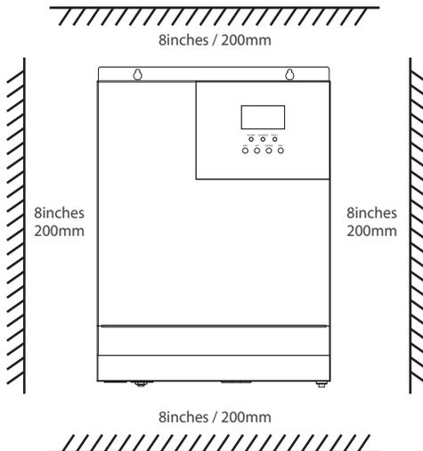
**Please Note:** While the Solar inverter has fans for cooling, this installation location optimal for natural convection cooling will improve the overall efficiency .
