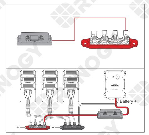
5. Attach the ring terminal of the other end of fuse cable to the Positive Busbar and tighten the wire retaining bolt with a wrench.
