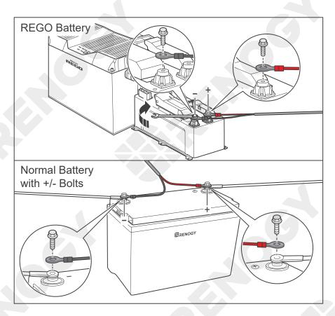
2. Connect the voltage sensor ring terminals to the positive and negative poles of the battery system.
