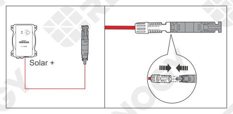
Connect the positive Solar Adapter Cable to the Solar Panel Fuse.
