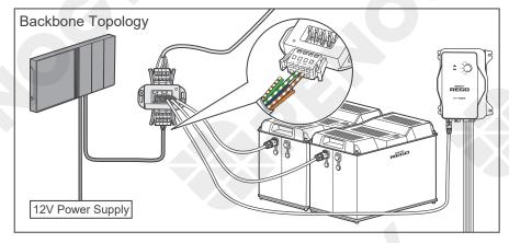
1. Replace the terminated drop tap at either end of the RV-C bus with the Common Drop Tap (not included). Secure the bare wires of the Drop Cable (not included) onto the terminal block plug of the Common Drop Tap following the terminal block plug pinout. Plug the Drop Cable to the RJ45 port of Renogy ONE.
