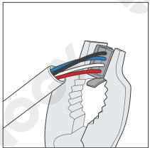
2. Squeeze the crimp areas of the Drop Plugs with the Split Joint Pliers.
