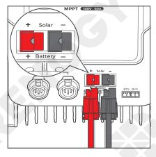
5. For the Solar terminal, align Anderson PP75 connectors of the Solar Adapter Cable to the correct orientation and polarity.
