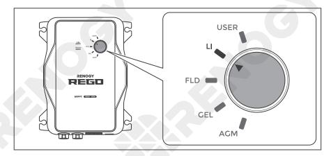
4. If the battery is Lithium Battery, turn the knob to LI.
