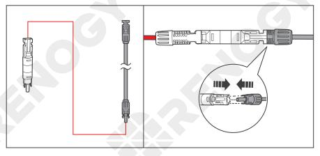
3. Connect the other end of the fuse cable to the Solar Panel Extension Cable.
