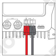
Insert the Anderson connectors into the Battery terminals.
