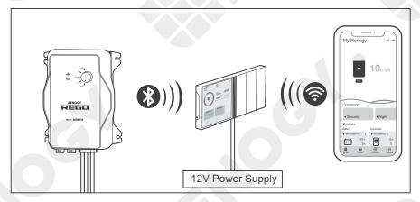
Connect the charge controller to the Renogy ONE (sold separately) through Bluetooth, and pair the Renogy ONE with the DC Home app through Wi-Fi. Monitor the charge controller on the Renogy ONE or the DC Home app.
