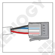
1. Insert the bare wires of the Drop Cables (sold separately) all the way into the wire ports of the Drop Plugs (not included) following the Drop Plug pinout. The red PS+ wires go to pin 1, the white CAN\_H wires go to pin 2, the blue CAN\_L wires go to pin 3, and the black PS- wires go to pin 4.
