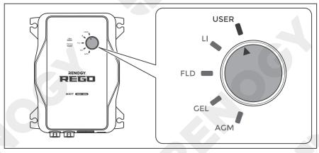
5. If multiple parameters of the battery need to be programmed, turn the knob to USER to enter the user mode.
