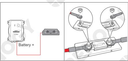
4. For your safety, it is recommended to use a battery fuse (80A). Connect the positive Battery Adapter Cable to one end of the battery fuse, and then connect the other end to the fuse cable.
