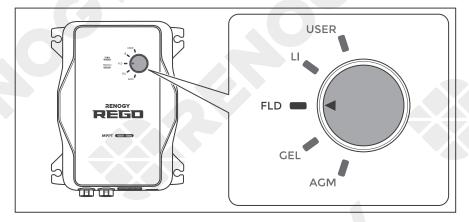
3. If the battery is Flooded Battery, turn the knob to FLD.
