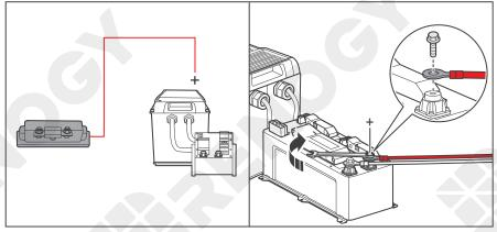
3. Attach the ring terminal of the positive Battery Adapter Cable (output) to the positive bolt of the battery and tighten with a wrench.
