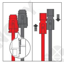
2. Bind the Anderson connectors by sliding the side grooves.
