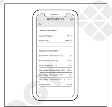
6. In this interface, you can customize multiple parameters of the battery. When the parameters are modified, **Setting Success** appears on the interface, indicating that the parameter setting is completed.
