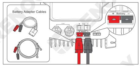
For the Battery terminal, align the Battery Adapter Cable's Anderson PP75 connectors to the correct orientation and polarity.
