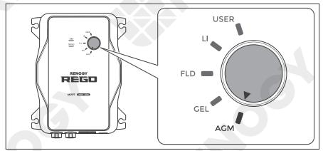
1. If the battery is AGM Battery, turn the knob to AGM.
