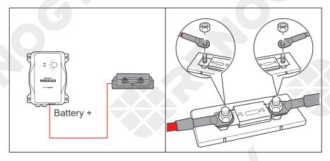
2. For your safety, it is recommended to use a battery fuse (80A). Connect the positive Battery Adapter Cable (output) to one end of the battery fuse, and then connect the other end to the positive bolt of the battery.
