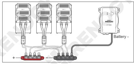
3. Connect the negative ring terminal of the Battery Adapter Cable to the Negative Busbars and tighten the wire retaining bolt with a wrench.
