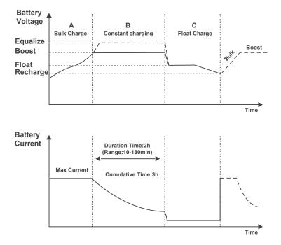
**Bulk Charge:** This algorithm is used for day to day charging. It uses 100% of available solar power to recharge the battery and is equivalent to constant current. In this stage the battery voltage has not yet reached constant voltage (Equalize or Boost), the charger operates in constant current mode, delivering its maximum current to the batteries (MPPT Charging).
